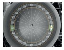
in which the two preset temperatures are respectively 15°C and 40°C, each sector represents an increment of 2.27°C.
